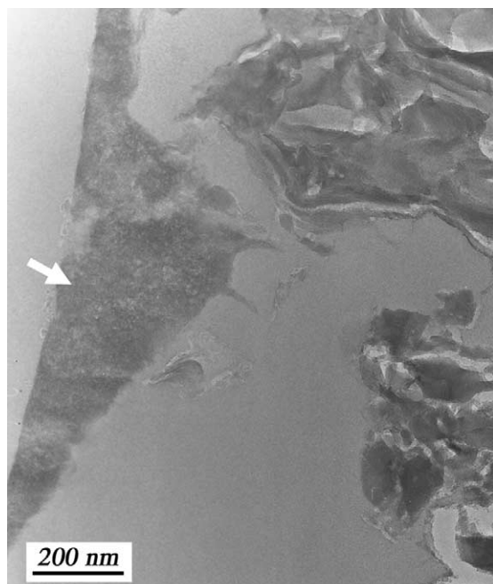
Fig. 9. TEM image of ferrihydrite and jarosite from the floodplain at Kohr's Bend (sample KB-2). The ferrihydrite, the wedge on the left side of the image denoted by the arrow, is the two-line variety with small amounts of Mn, Pb, and As present (see Hochella et al. (in press) for identification details). Jarosite crystals make up the right side of the image.
