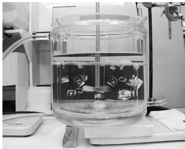
FIGURE 1. Water-jacketed crystallization vessel with variable-speed stirrer for alum experiments.
