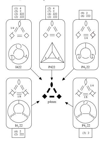
Figure 2.7. Space group orbifolds from point group 422 and plane group p4mm.
